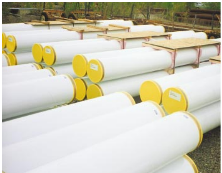
The TP-pipes were supplied on pallets. Each pipe is packed separately and is therefore protected against transport damage.
